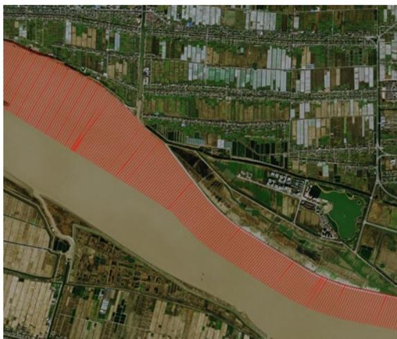
Figure 1. Layout of sounding lines
