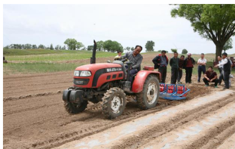
Figure 2. 5-wheel-combination machinery hill-drop buckwheat 图 2. 5 轮组合机穴播荞麦
