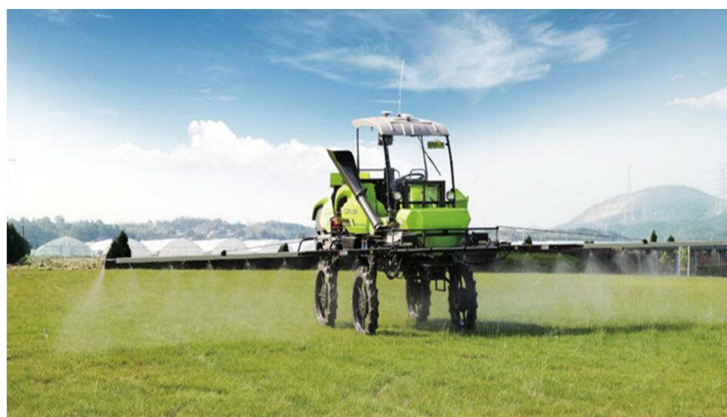
Figure 5. Zoomlion Valley King 3WP-600HA self-propelled boom sprayer 图 5. 中联谷王 3WP-600HA 自走式喷杆喷雾机
