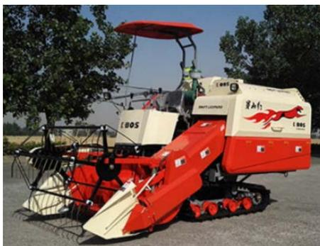
**Figure 3.** 4LZD-1.6Z soybean combine harvester
