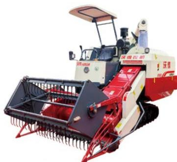
**Figure 2.** 4LZD-2.6AQ soybean harvester
