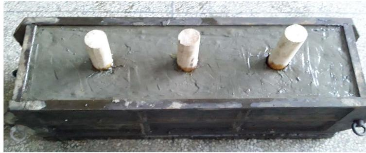
Figure 10. Preformed hole
