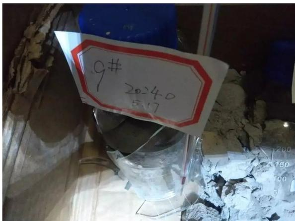
**Figure 3.** Breaking situation of glass bottle 9# in the 210<sup>th</sup> min
