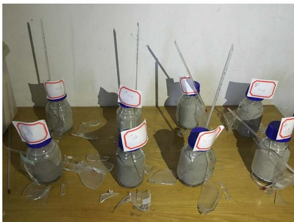
**Figure 2.** Situation of breaking glass bottle 1#-8# in the 90<sup>th</sup> hour
