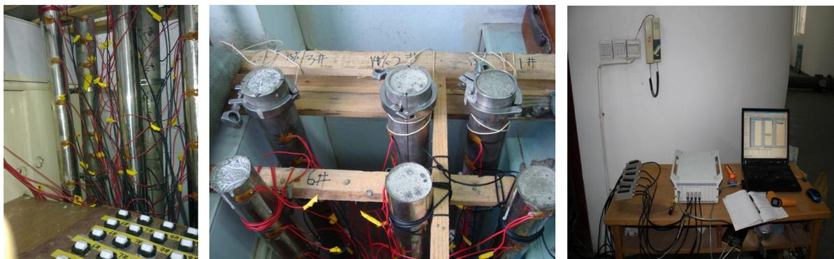
Figure 8. Experimental facility and test system for expansion pressure testing
