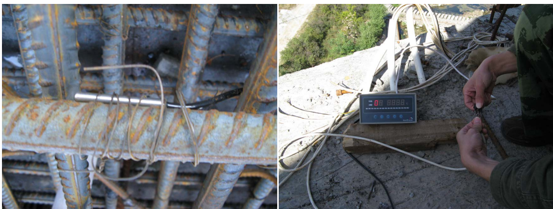
Figure 5. Field temperature acquisition. (a) Thermal resistance temperature sensor; (b) temperature measurement acquisition module
