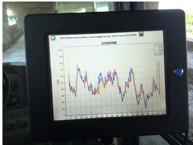
Figure 12. Control terminal displays CMV curve
