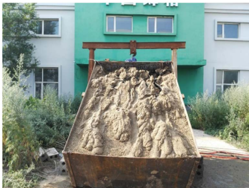
Figure 5. Specimen after water flow erosion 图 5. 水流冲刷后试件
