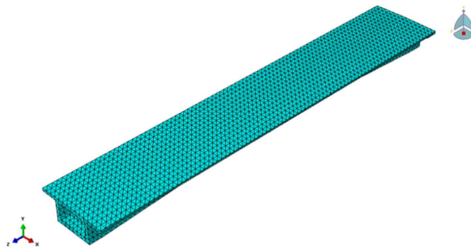
Figure 11. Finite element model of reinforcement concrete beam
