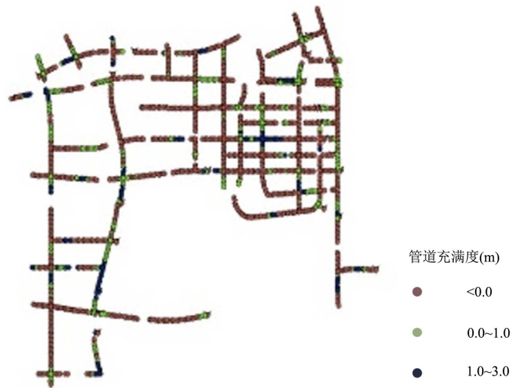
Figure 7. Overflow distribution map of inspection well 图 7. 检查井溢流分布图
