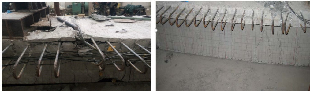
Figure 6. Photos of the ultimate failure of the test beam 图 6. 试验梁最终破坏照片
