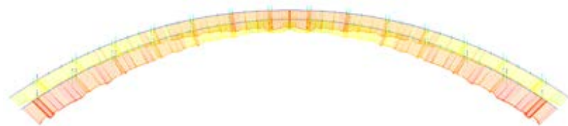
Figure 21. Stress diagram of main arch during service 图 21. 主拱服役全过程应力情况示意图
