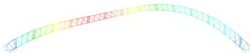
Figure 14. Deformation diagram of main arch after installation of the seventh span 图 14. 第七跨安装完主拱变形示意图
