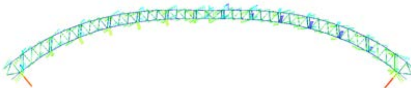
Figure 17. Schematic diagram of main arch internal force after installation of the whole bridge (shear force)
