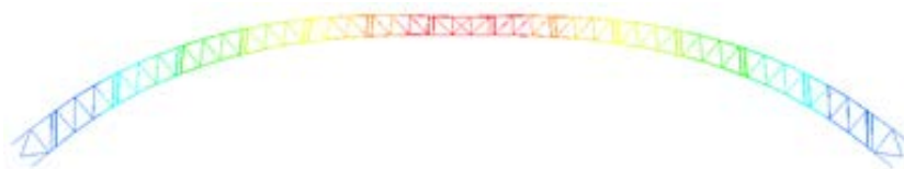
Figure 15. Deformation diagram of main arch after installation of the whole bridge 图 15. 全桥安装完主拱变形示意图
