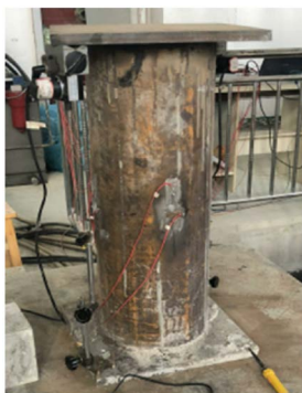
Figure 3. Test device diagram of the strain gauge 图 3. 试验装置图
