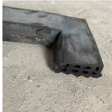
Figure 10. Schematic diagram of hollow corner of shield tunnel sealing gasket 图 10. 盾构隧道密封垫空心转角示意图
