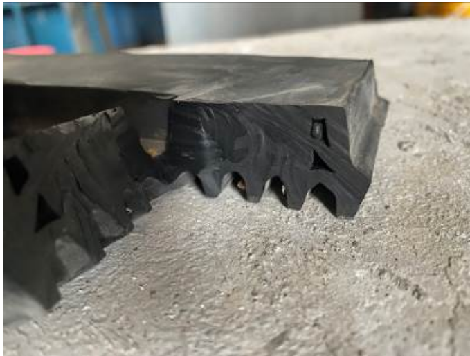
Figure 1. Schematic diagram of solid corner of gasket
