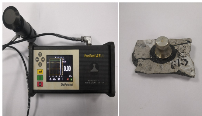
Figure 1. PosiTest AT-A adhesion tester (left), test sample (right) 图 1. 全自动附着力测试仪(左)、试验样例(右)
