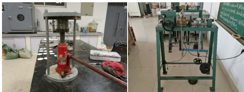
Figure 2. Direct shear test in room 图 2. 室内直剪试验
