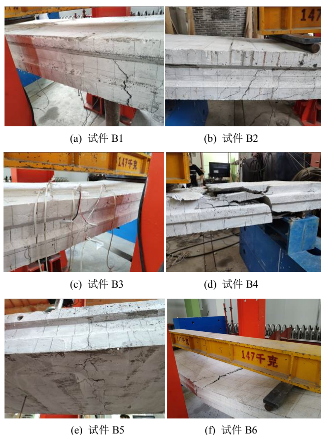
Figure 3. Failure modes of specimens 图 3. 试件破坏形态
