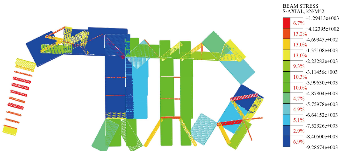
Figure 10. Internal support stress diagram 图 10. 内支撑应力图
