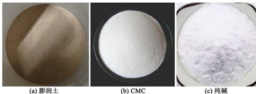
**Figure 1.** The mud material used in the test
