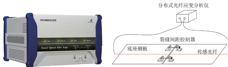
Figure 3. Diagram of crack measuring device 图 3. 裂缝测量装置图
