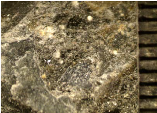
G Group II: topography of 28d Grain size of the coarse aggregate: 16 mm, 4.75 mm, 2.36 mm. Scale: 2.5:6.5:1 G 第二组 28d 粗骨料粒径: 16 mm, 4.75 mm, 2.36 mm。比例: 2.5:6.5:1
