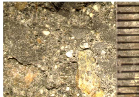
D Group IV: topography of 3d Grain size of the coarse aggregate: 16 mm, 4.75 mm, 2.36 mm. Scale: 1:1:3:1 D 第四组 3d 粗骨料粒径: 16 mm, 9.5 mm, 4.75 mm, 2.36 mm。比例: 1:1:3:1
