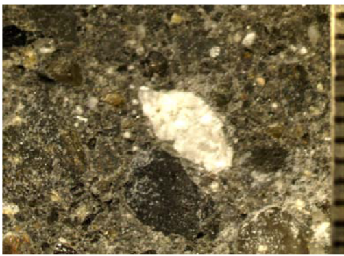
J Group V: topography of 28d Grain size of the coarse aggregate: 19 mm, 16 mm, 9.5 mm, 4.75 mm, 2.36 mm. Scale: 1:1:1:3:1 J 第五组 28d 粗骨料粒径: 19 mm, 16 mm, 9.5 mm, 4.75 mm, 2.36 mm。比例: 1:1:1:3:1
