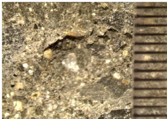
C Group III: topography of 3d Grain size of the coarse aggregate: 16 mm, 4.75 mm, 2.36 mm. Scale: 2:7:1 C 第三组 3d 粗骨料粒径: 16 mm, 4.75 mm, 2.36 mm。 比例: 2:7:1
