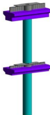
Figure 13. Concrete-filled steel tube column 图 13. 钢管混凝土立柱
