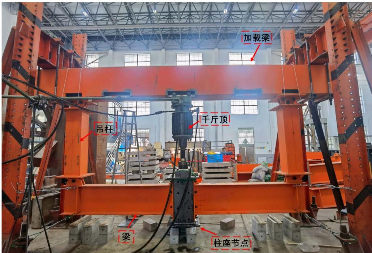
Figure 2. Loading device of fatigue test
