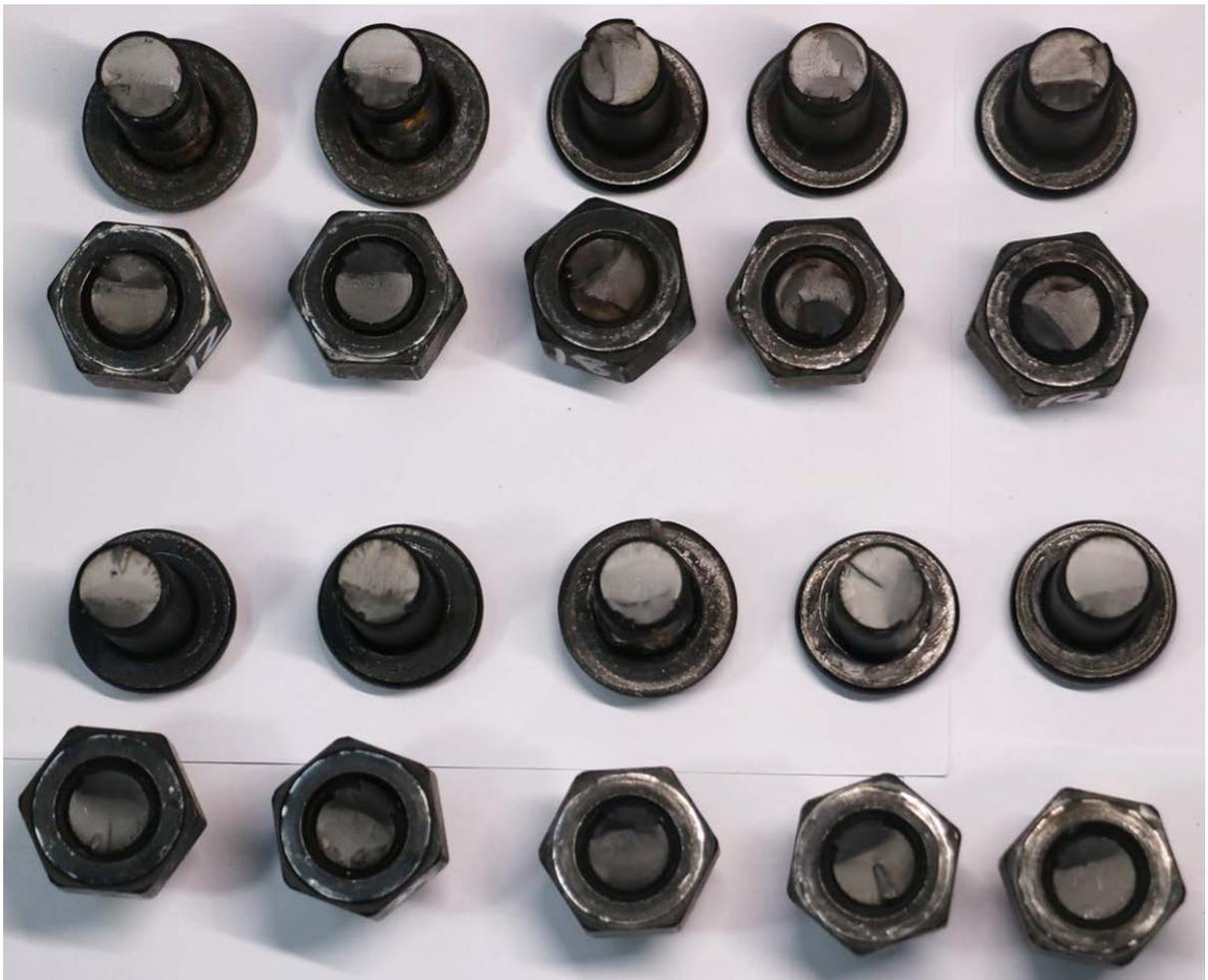
Figure 5. Real picture of high-strength bolt after damage
