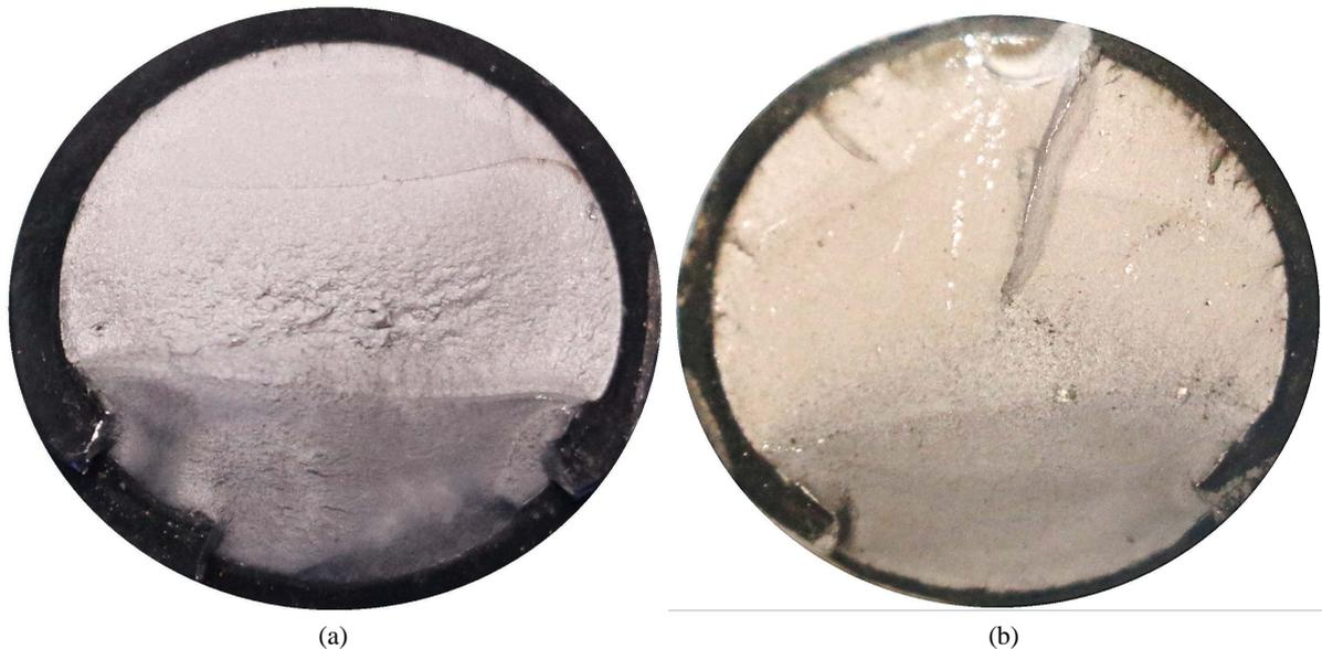
Figure 6. The fracture of M20 high-strength bolt
