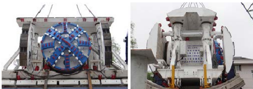
Figure 5. Mobile segment prestressing support system 图 5. 移动式管片预应力支撑系统
