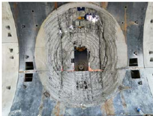
Figure 3. Tapered discs for simulating experimental cutting results 图 3. 锥形刀盘模拟试验切削效果
