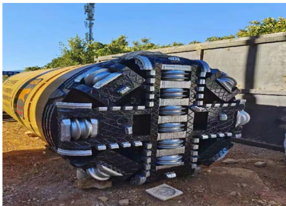
Figure 2. Pipe jacking machine
