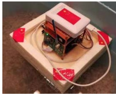
Figure 3. Automatic device for spatial coordinates of underwater riverbed
