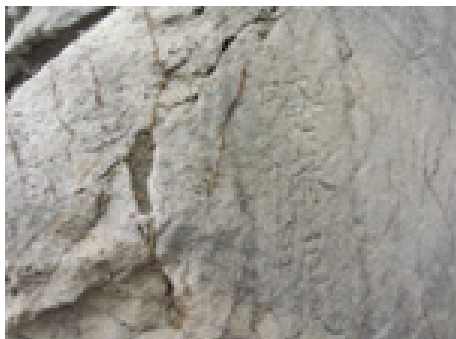
Figure 4. Rain scratches on the surface of Moya stone inscriptions 图 4. 焦山摩崖石刻表面的雨痕
