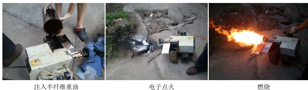
Figure 4. Boiler burner test results of hemicellulose crude oil 图 4. 半纤维素重油锅炉燃烧试验结果
