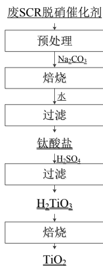
Figure 5. Dry recovery process flow chart 图 5. 干法回收工艺流程图
