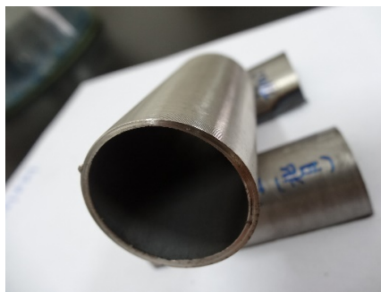
Figure 4. High temperature superheater tube 图 4. 高温过热器管
