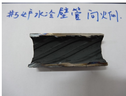
Figure 2. Water cold wall tube to the inner surface of the fire of #5 unit 图 2. #5 机组水冷壁管向火侧内表面
