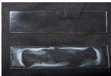
Figure 7. Comparison chart of changes in defluorination agent before and after reaction 图 7. 脱氟剂反应前后整体变化对比图
