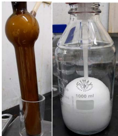
Figure 3. Absorbent liquid is converted into bubble overflow
