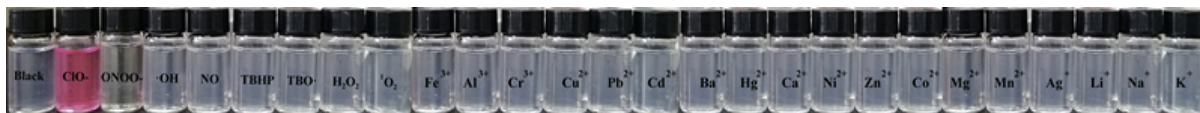
Figure S1. Photos of the probe TPE-RhB in ethanol/water (50 \mu\text{mol/L} , v/v, 1/1, PBS, pH 7.4) after adding different ROS/RON and metal ions (8 equiv.) under natural light
