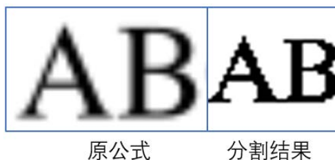
Figure 8. Conglutination caused by image processing 图 8. 图像预处理造成的字符粘连示例
