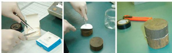
Figure 1. Measurement of soil water characteristic curve
