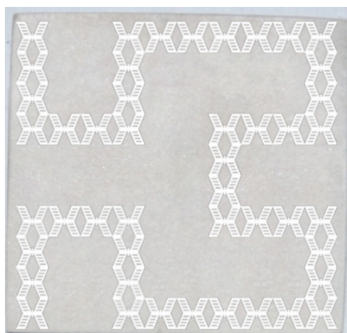
Figure 4. The sample photo of high compatibility fractal array bionic antenna 图 4. 高兼容性分形阵列仿生天线样品照片
