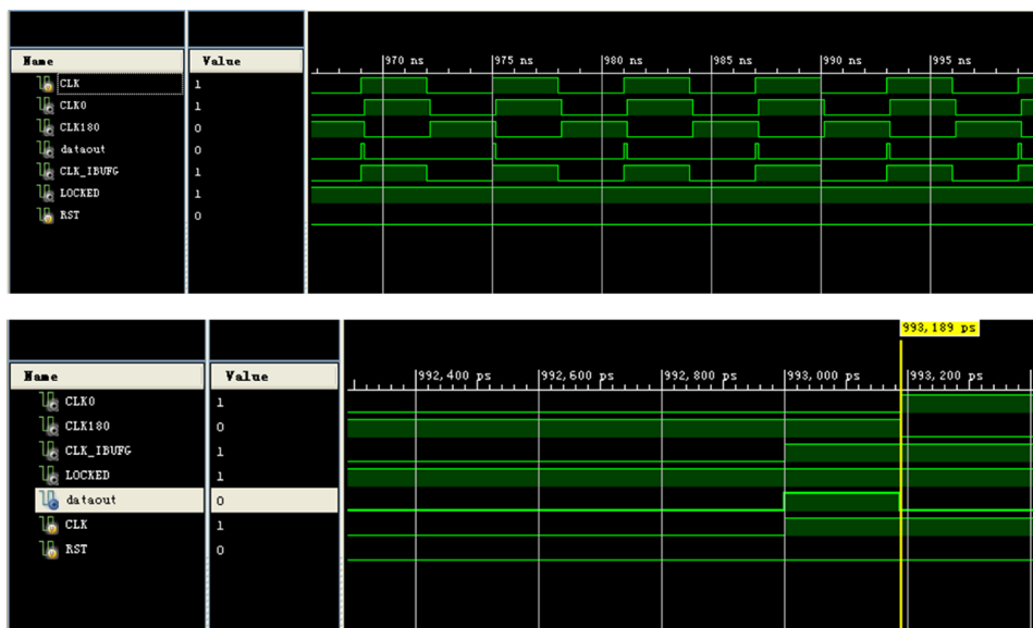
Figure 10. Simulation results of narrow pulse generation in digital circuits based on DCM
