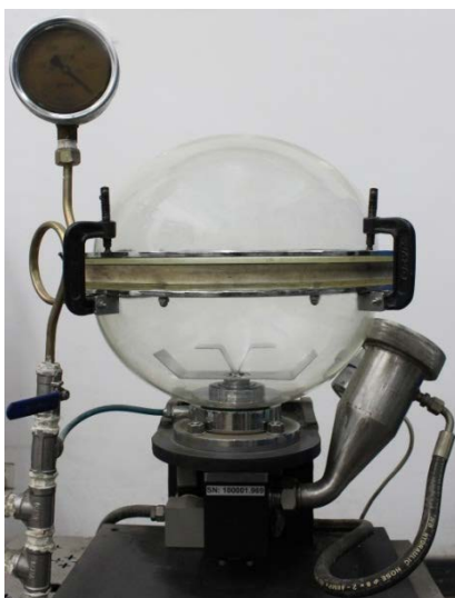
Figure 1. The transparent Siwek 20 L test chamber
