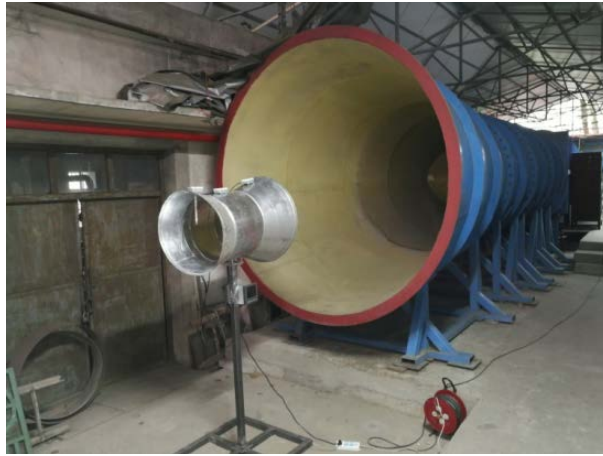
Figure 3. Test system of the air duct 图 3. 聚风筒实验测试系统
