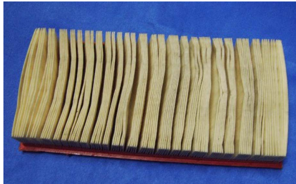
Figure 7. Deformation state of paper filter element after life cycle test 图 7. 寿命测试周期完成后纸质滤芯变形状态
