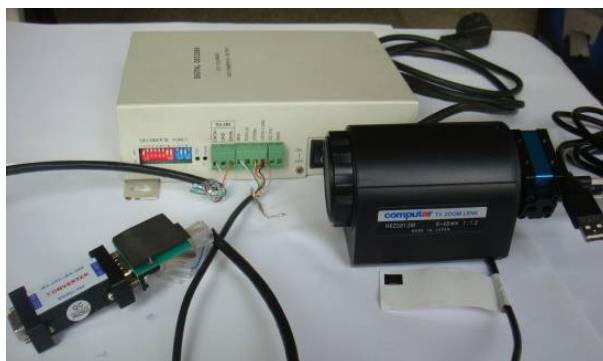
Figure 6. Hardware connections of acquisition system 图 6. 采集系统硬件连接
