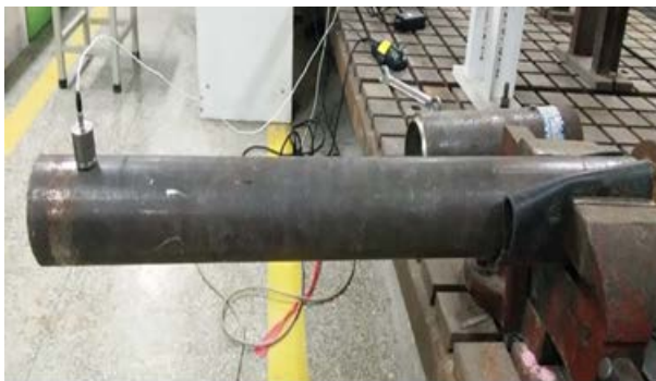
Figure 9. Test bed for stainless steel lined steel pipe
