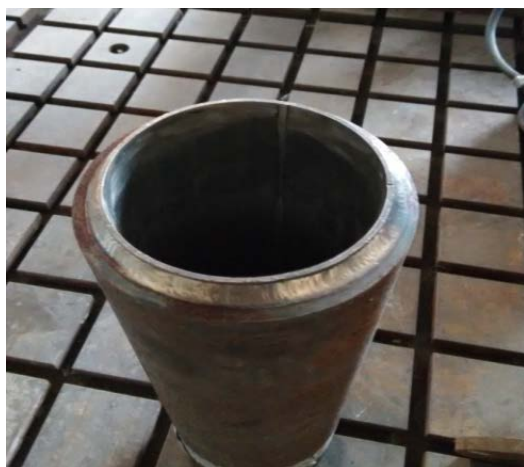
Figure 6. Stainless steel lined steel pipe 图 6. 内衬不锈钢钢管
