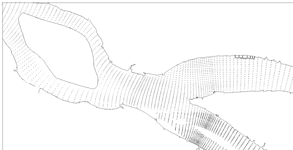
Figure 7. Distribution of Velocity field in spring ebb 图 7. 大潮落急流速场分布
