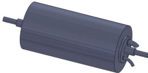
**Figure 1.** The 3D model of the conducting oil heating cylinder
