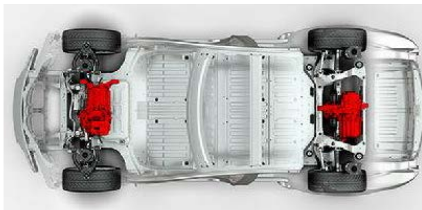
Figure 4. Tesla's perspective (battery in the middle of the body)
