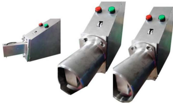
Figure 7. Auxiliary measuring parts replacement process 图 7. 测量辅件更换过程
