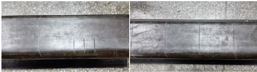
Figure 2. Artificial defects rail specimen 图 2. 人工缺陷钢轨试件
