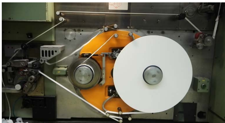
Figure 12. Schematic diagram of ZJ17 cigarette paper recovery device assembly 图 12. 卷烟纸回收装置安装示意图
