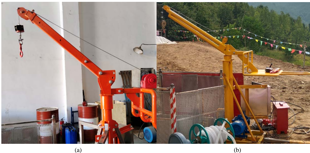
Figure 1. (a) Boom retractable crane; (b) Fixed boom length crane 图 1. (a) 吊臂可伸缩起重机; (b) 吊臂长度固定起重机
