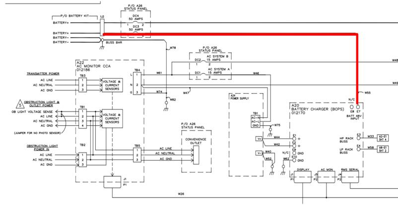
Figure 3. BCPS and battery connection circuit diagram
