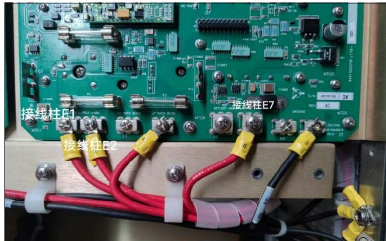
Figure 4. BCPS board binding posts
