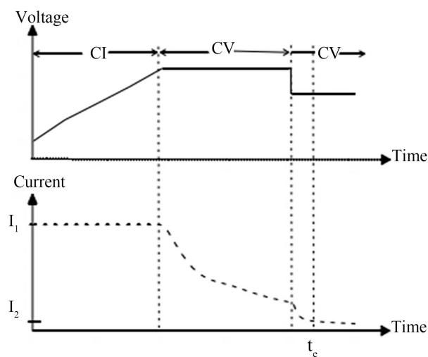
**Figure 8.** Three-stage charging method voltage and current change curve
