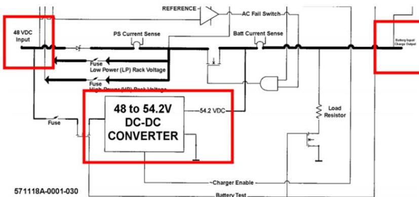
Figure 5. BCPS module block diagram
