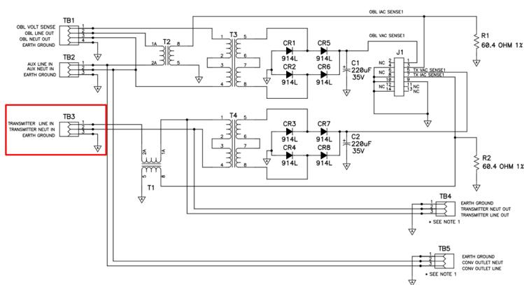
**Figure 1.** AC MONITOR circuit diagram
