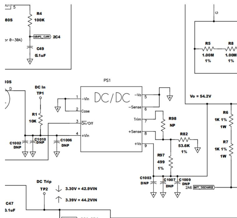
Figure 6. BCPS boost module circuit diagram
