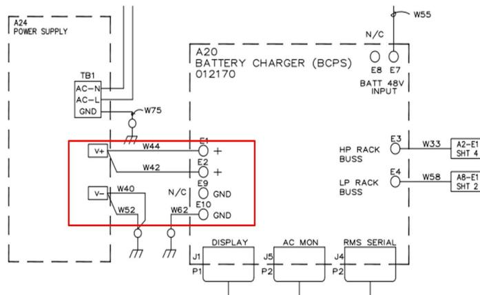
**Figure 2.** BCPS and Power Supply circuit diagram
